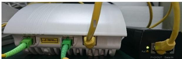
1. Connecting PoE injector to AC power
