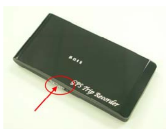
Power off (Before)
