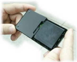
Step 2 Open the cover of battery
